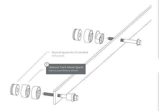
Black bumpers included in Trolley Stop Track Mount Kits are designed to stop the door panel. Position them at end of track, or where you want door panel to stop.
