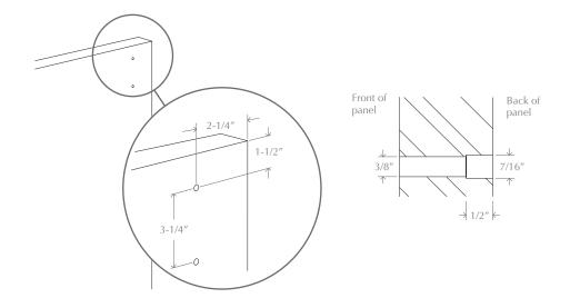
Install safety stop to top of door panel.
