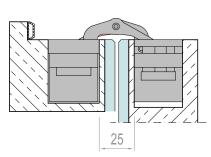
Section of Wood Frame-Door Installation
