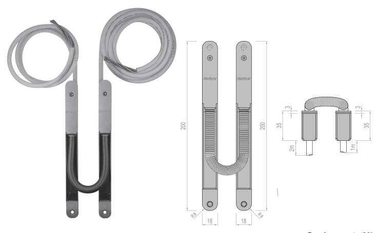
Concealed 8-pole, electric wire connection for permanent power transfer to the door leaf. Connector's components are mortised into door and frame. The wire on one side can be separated for easier installation.
