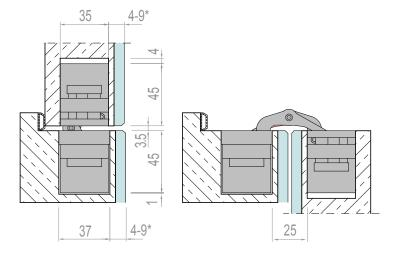
Section of Wood Frame-Door Installation
