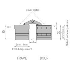
3-D adjustable concealed hinge for flush doors. Hinge leaves are mortised into the frame and door. Magnetically fixed coverplates provide installation without visible fasteners.
