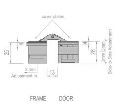
3-D adjustable concealed hinge for flush doors. Provides increased throw for optimized milling tolerances. Hinge leaves are mortised into the frame and door. Magnetically fixed coverplates provide installation without visible fasteners.
