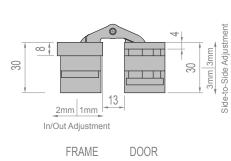
3-D adjustable concealed hinge in **Solid 304 Series Stainless Steel** for enhanced corrosion resistance. Recommended for exterior and marine environments.
