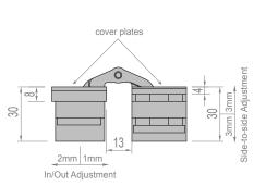
3-D adjustable concealed hinge for flush doors. Hinge leaves are mortised into the frame and door. Magnetically fixed coverplates provide installation without visible fasteners.
