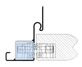
For securing PIVOTA® DX concealed hinges to steel frames; the receiver can be adapted to the respective profile of the steel frame.
